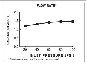
1.5 gpm/5.7 L/min. FLOW RATE
